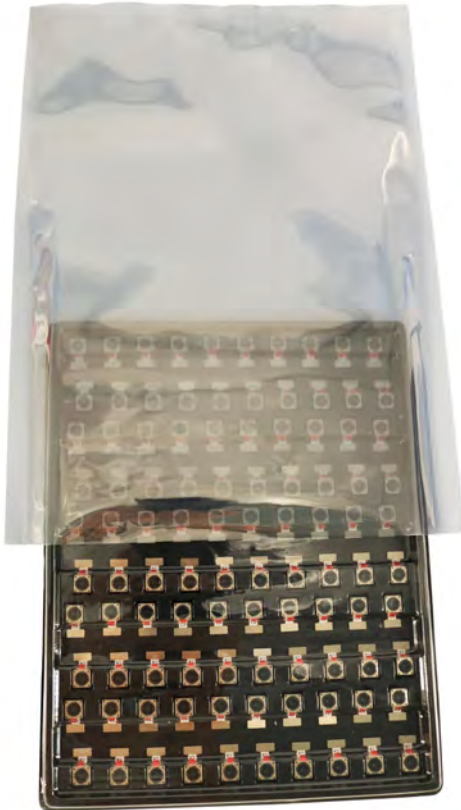
Place Tray into Anti-Static Bag
